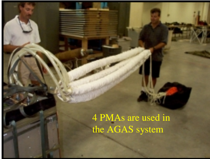
Figure 3. Pneumatic Muscle Actuators (PMAs)
