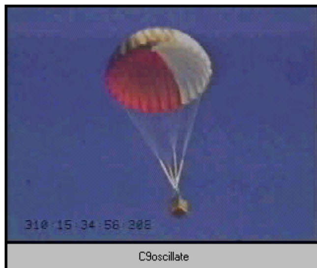
Figure 22. Parachute Oscillations (video clip)
